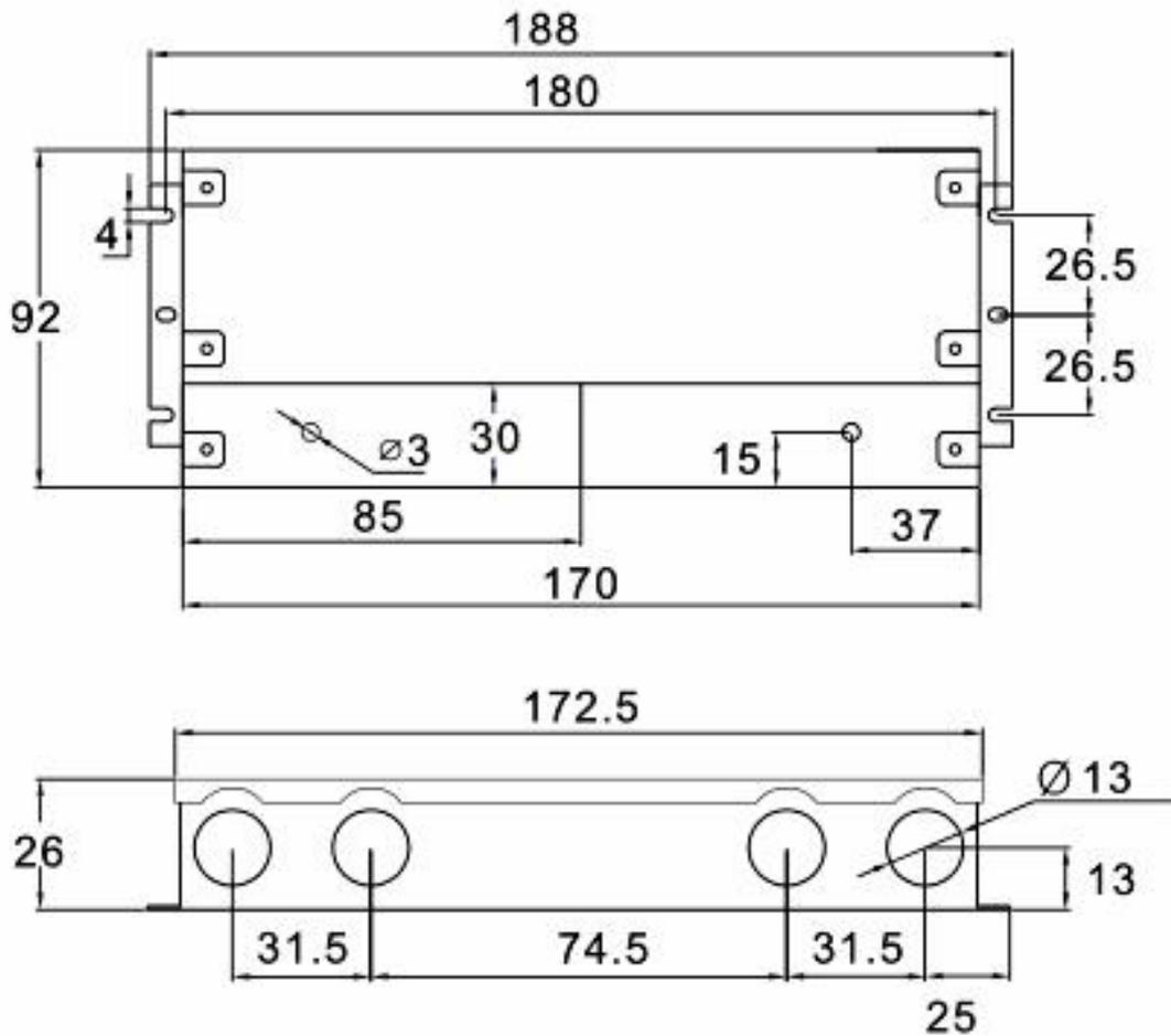
※Input:18AWG Black and White to be connected to AC L and N ,Green wire go ground,
