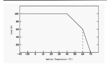
Load carried in accordance with the load derating curve, according to the ambient temperature derating, in order to extend the service life
